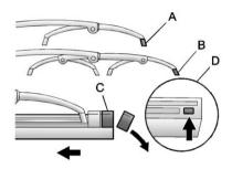
Slide the insert (D), notched end last, into the end with the two blade claws (A). Slide the insert all the way through the blade claws at the opposite end (B). The plastic caps (C) will be forced off as the insert is fully installed.
